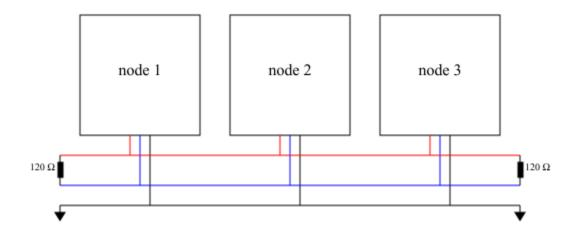
Messages are transmitted on the CAN bus as a series of bits. 0 bits (called dominate bits in CAN terminology) are signaled by applying a differential voltage to the CAN high and low bus lines. 1 bits (called recessive bits in CAN) are signaled by not driving the bus and allowing the terminating resistors to reduce the differential voltage to zero.
