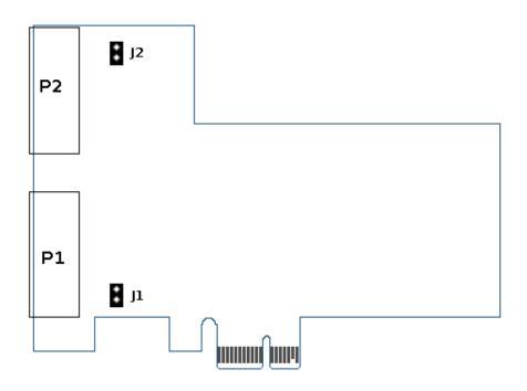
The card uses a single lane PCI express connector to interface with the host computer. The card can be installed in any PCI express slot on the host PC, both single lane slots and multi-lane slots will work equally well.
